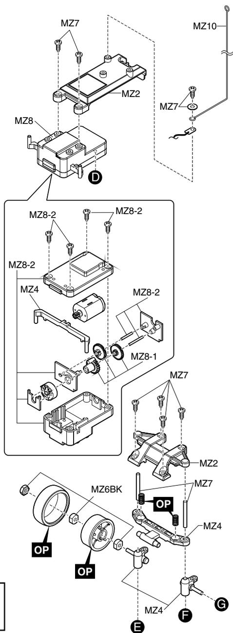
▶ When using Spare Parts MZ-10, bend it as illustrated and then install.
