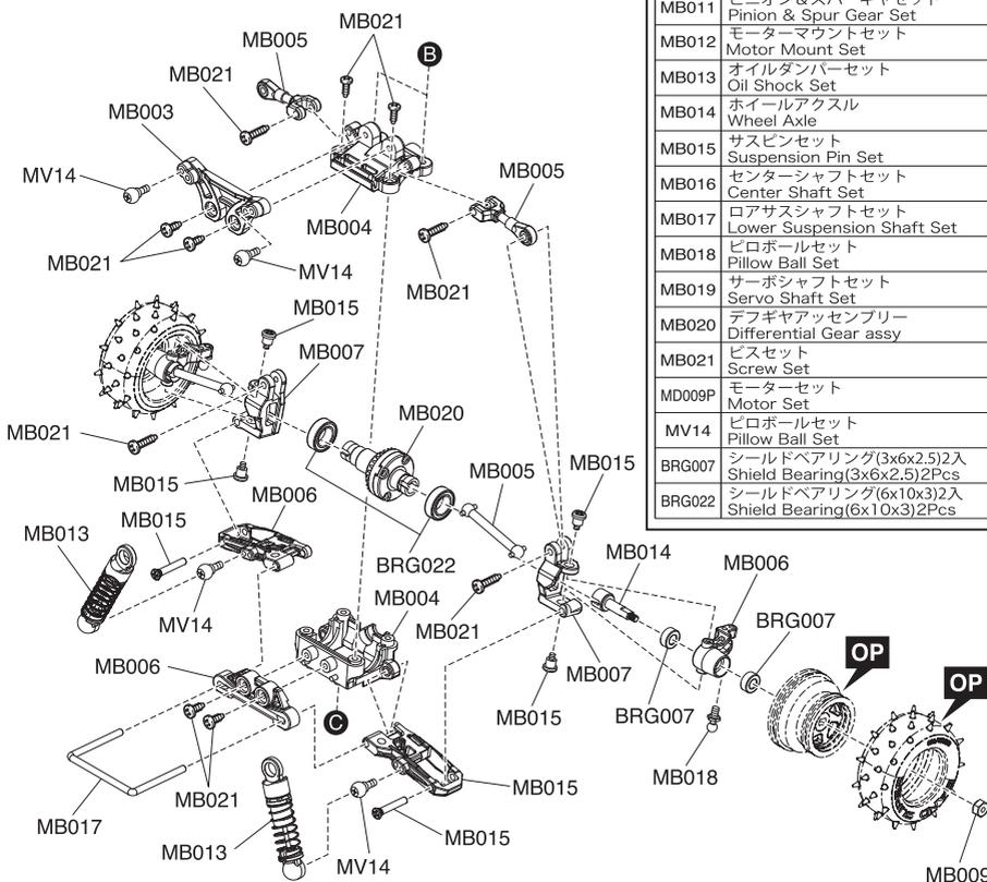
▶ The optional parts should be used for the parts marked with **OP**.
