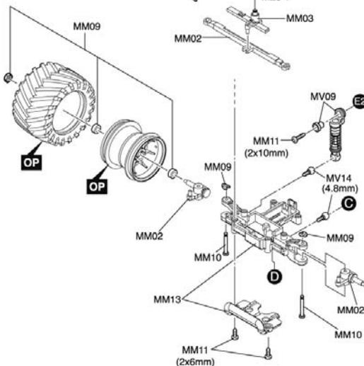
▶ The optional parts should be used for the parts marked with **OP**.
