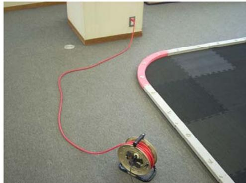
A. When the power cord is coiled, bound or in reel, noise is likely to occur. Always have the cord stretched. If cord-reel is being used, pull out the entire cord.
