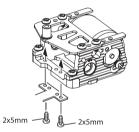
▶ シャシーへの取付けは 内側の2本のビスで固定。 Install screws through the inside holes ofthe plate when attaching the motor mount assembly to the chassis.
