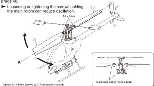
If both rotors are unbalanced, there may be some vibration in the direction of the elevator. If balance is not easy to adjust and there is vibration in the direction of the elevator, firmly fix (1) so they are in a straight line.
