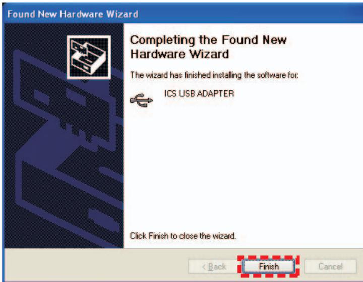
8. After completing installation of the ICS USB Adapter, perform the installation of the USB Serial Port driver.
