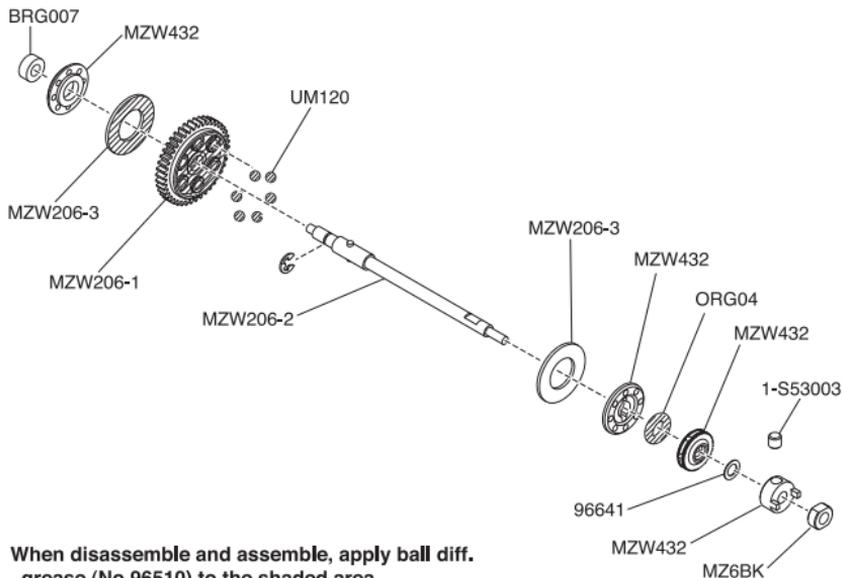
When disassemble and assemble, apply ball diff.
