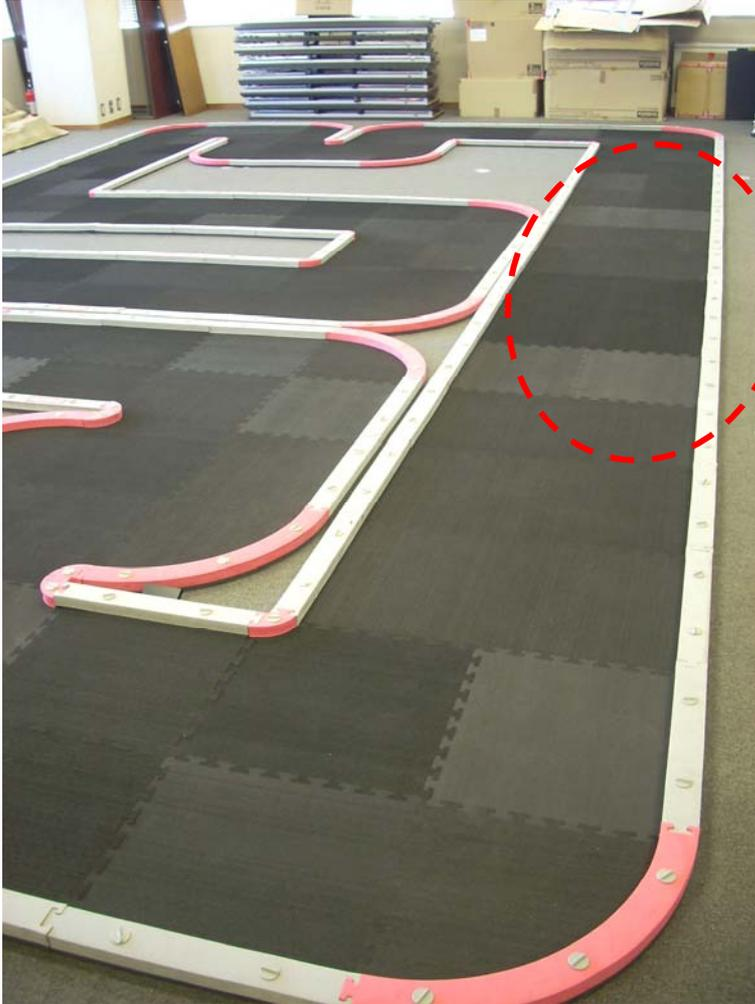
2. Area with gap or where crashes occur frequently usually lift the chassis and disable proper capturing of signals.
