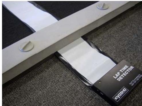
3. Cover the receptor with the plastic folders. Have the edges of the plastic under the walls of the circuit.
