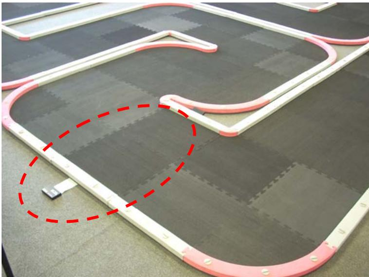
Within the perimeter of about 20cm of the receptor, there should be no metallic object.
