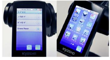
4. Choose "Drone Racer" then the icon of "Mode setup" will change to DRONE RACER.
