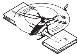
Motor will not turn if Throttle Stick is not all the way down or Throttle Trim is not center.
