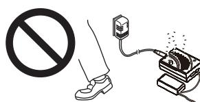
Do NOT charge in direct sunlight or in places with high temperatures.
