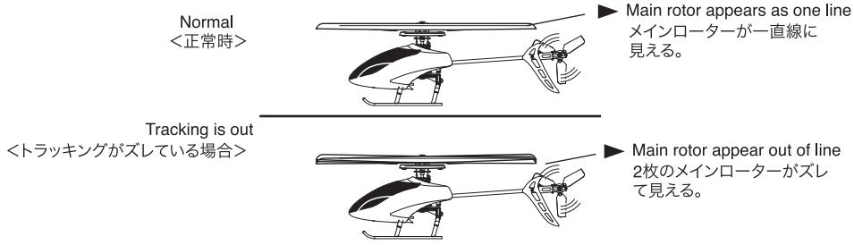
**3** Adjust tracking according to the following process.
