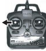
Move the Throttle Stick slightly upwards and the tail motor and main motor will start to turn.
