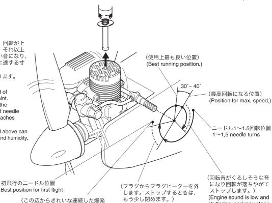
音「ピーン」で高音になってきます。) (At about this point, the engine should give a sustained high pitched sound.)
