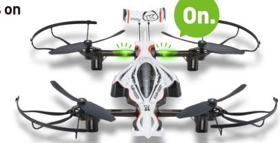
To change to the flight mode, turn the steering wheel fully to the left and simultaneously apply full forward throttle by pulling the trigger towards you. The LEDs on the rear arms change to red, indicating the
