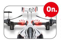
Red LEDs mean the Drone Racer is ready for flight. After 5 seconds without any activity, however, the safety function will automatically re-activate and you'll need to activate the flight mode again.
