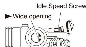
Unscrew the Idle Speed Screw to decrease rpm.
