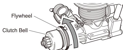
\* Idling RPM is when the flywheel is rotating while the clutch bell remains static.
