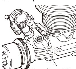
Tighten screw so it protrudes 0.4 - 0.5mm.
