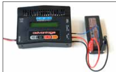
Car battery connection (with SLPB balancing wire)
