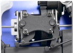
extra dimension of control where power is balanced front-to-rear, in addition to the side-to-side differential action already provided by the front and rear diffs.
